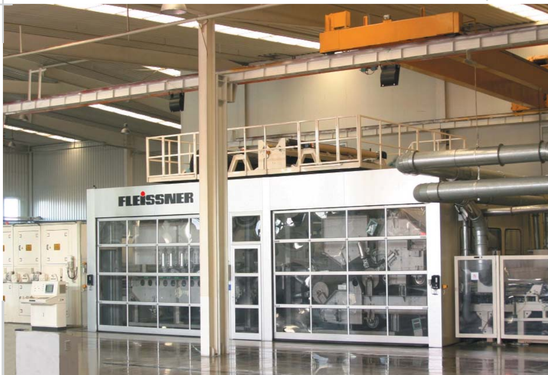
Fleissner AquaJet of 3.6 m working width for the production of two layer products and special wipes with unwinder on top.
