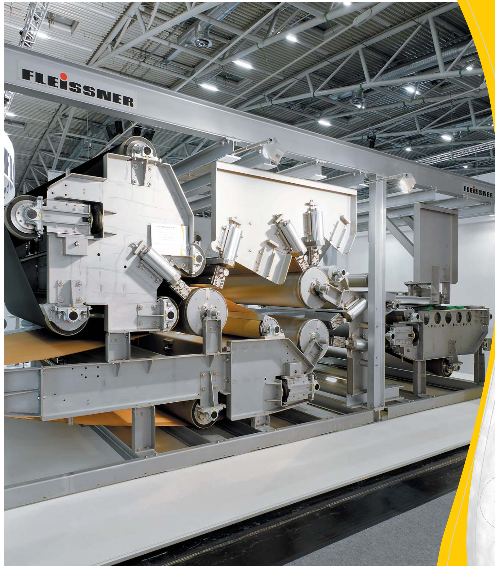
Fleissner AquaJet of 3.6 m working width for a two layer product of medium weight consisting of an electro spun nanoweb and a polyester (splittable fiber type) web. Applications are artificial leather and premium sports textiles.
